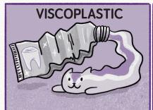
A plastic solid at low stress, and a viscous liquid at high stress
